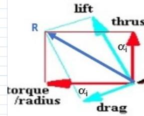
$$dt(r, \theta, u) := dl(r, \theta, u) \cdot \cos(\alpha(r, \theta, u)) - dd(r, \theta, u) \cdot \sin(\alpha(r, \theta, u)) \quad dt\left(10 \text{ ft}, 10 \text{ deg}, 5 \frac{\text{ft}}{\text{sec}}\right) = 165.513 \frac{\text{lbf}}{\text{ft}}$$
